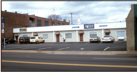
Building heights in Downtown Russellville should not exceed three stories. The front setback above is too deep, and parking should not be in front of the building.
